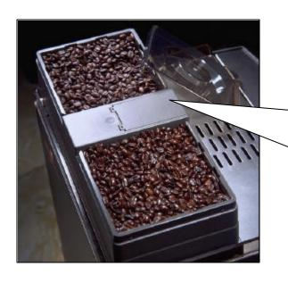
There is an inlet opening, covered with a lid, located between the two hoppers. Cleaning tablets should only be dropped into this opening for use during the end-of-day cleaning procedure. The cleaning program is geared toward the use of the Schaerer tablets only. Do not use powder or tablets made by any other manufacturer!
