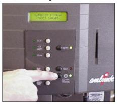
The machine will run a cleaning cycle for approximately 5 minutes. During this cycle the selection of beverages is locked. Once the cleaning cycle is finished the display will show the message: "select beverage".
