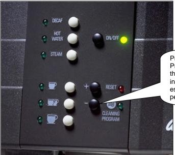
Press and hold the 'Cleaning Program' button for 4 seconds and the machine will go through a brief internal hot water flush. This is especially effective immediately after peak dispensing hours.
