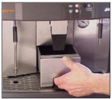
2. Remove the coffee spout and take out the metal shield above the grounds bin.
